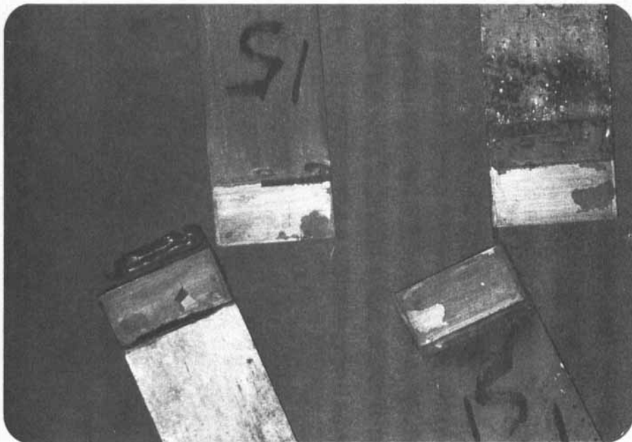
FIGURE 10 Corroded aluminium joints (after 60-days immersion in sodium chloride solution). See Color Plate I.
